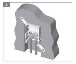
Please pay attention to a tension-free installation and the correct flow direction (supply flow left - see arrow mark!) when connecting the piping system. Reversely mounted connections cause valve noises and a bad control behaviour. Tension-free compression connection must also be guaranteed when the system is in operation, i.e. expansion loops or appropriate securing of the pipeline must be provided.
